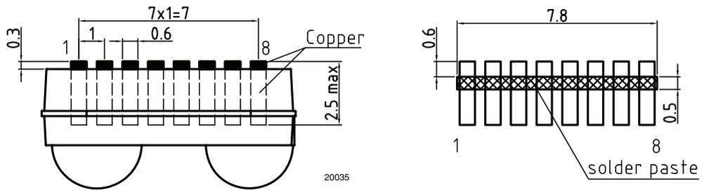
Figure 8. Recommended footprint for side view applications and solderpaste mask
