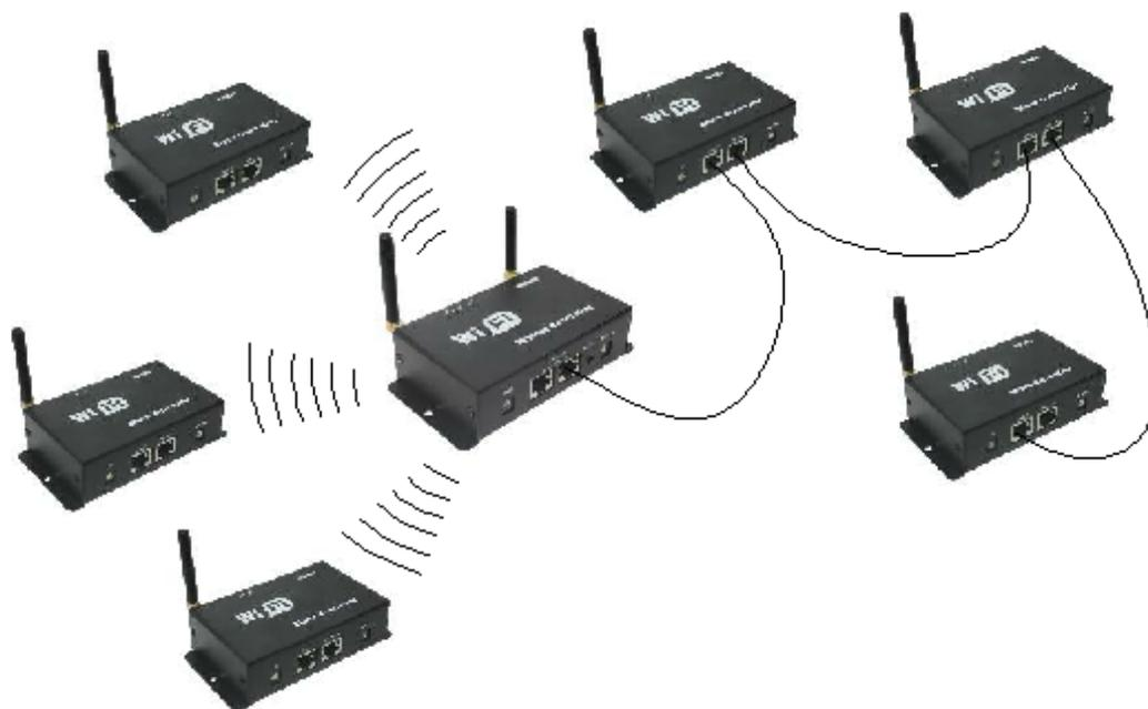
**Notice:** when use the wireless control, in order to achieve the best effect, the master should be placed in each slave control center position.
