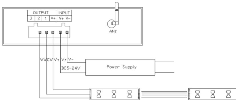
When connect three channels LED, you should put the Magic Color 1.0 software switch to CD mode to use, only under this mode, you can control the LED's color temperature, brightness and color temperature shortcut key settings. Color disk adjust the color temperature (meanwhile top left CW, WW numerical with change), brightness item adjust bright, "M" key set the special color temperature state.
