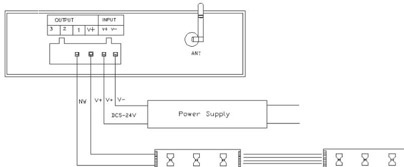
When connect one channel LED, you should put the Magic Color 1.0 software switch to DIM mode to use, under this mode, use color disk control the LED's brightness, Adjust process can be seen in the upper left corner NM numerical with change.
